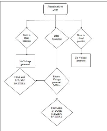
**Figure 1:** Illustrate the flow diagram for the generation of the electricity from the doors.
