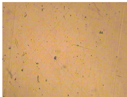
Figure 7: Corroded surface of 410-MN: 1.8 420-MN: 2.8 (Stainless Steel) in Murban.
