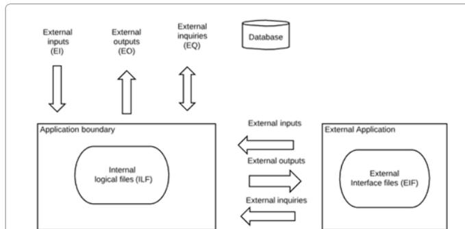
**Figure 1:** The boundaries of the myteam website for FPA-evaluation. The application boundary is defined as the boundary to the MYSQL database. The external application is taken as the PHP-source-code on the web-server. External inquiries (EI) are files with SELECT statements. External input are files with DML statements INSERT, UPDATE and DELETE. External outputs (EO) would be SMS and email services.
