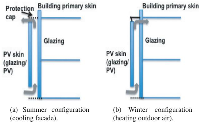
**Figure 1:** Operating principal of the double skin in addition to classical envelope function.
