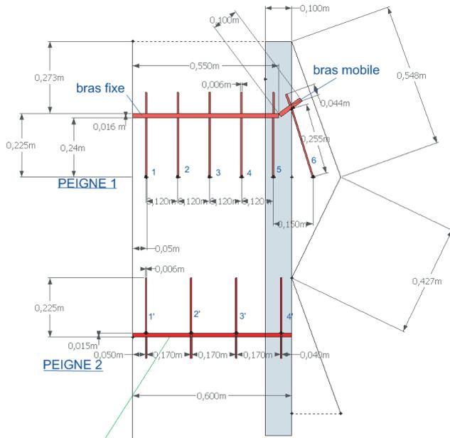
Figure 5: Thermocouples and velocity probes spatial repartition in the air gap.
