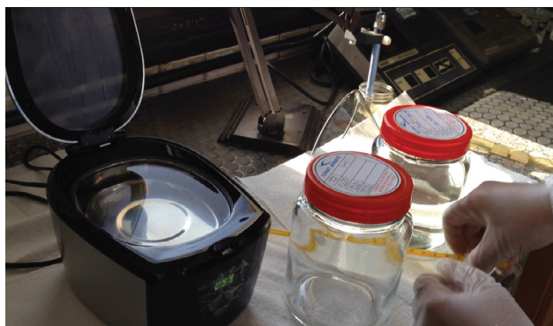
Figure 11: Shows fuel sample in the ultrasonic device in the microbiological fuel laboratory.
