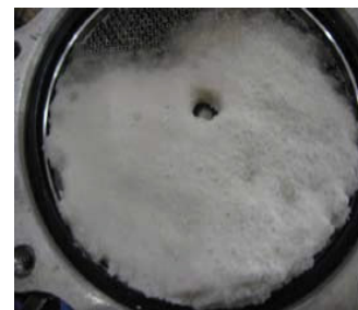
Figure 3: Shows fuel oil heat exchanger when water in fuel turning into ice crystals and restricting fuel flow source: (Aircraft Accidents Investigation Branch, 2010).
