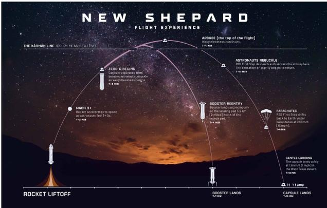
Figure 1: New Shepard flight trajectory.
