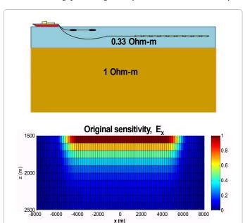
Figure 1: Top panel: Typical in-line towing configuration of sources and receivers for a marine towed streamer EM survey.
