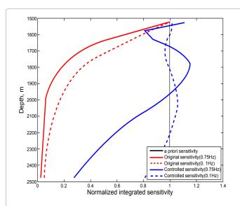
**Figure 4:** Plots of the original (red lines), a priori (black line), and controlled integrated sensitivities (blue lines), normalized by the maximum of the corresponding a priori sensitivity. The sensitivities are computed for a typical marine towed streamer EM survey configuration, shown in Figure 1 at frequencies of 0.75 Hz (solid lines) and 0.1 Hz (dashed lines).
