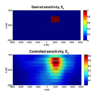
**Figure 3:** Top panel: Desired a priori sensitivity for a typical marine towed streamer EM survey configuration, shown in figure 1.
