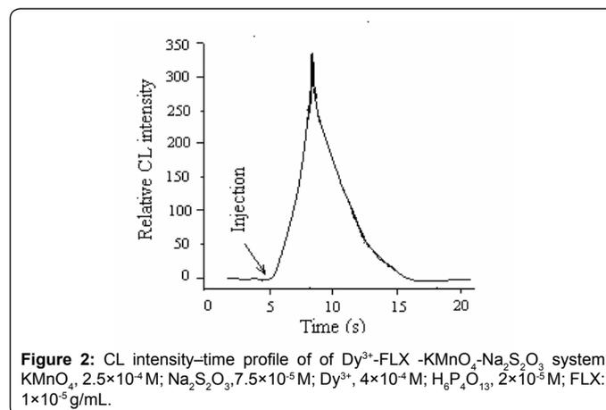
Figure 2: CL intensity-time profile of of Dy<sup>3+</sup>-FLX -KMnO<sub>4</sub>-Na<sub>2</sub>S<sub>2</sub>O<sub>3</sub> system KMnO<sub>4</sub>, 2.5 $\times$ 10<sup>-4</sup> M; Na<sub>2</sub>S<sub>2</sub>O<sub>3</sub>, 7.5 $\times$ 10<sup>-5</sup> M; Dy<sup>3+</sup>, 4 $\times$ 10<sup>-4</sup> M; H<sub>6</sub>P<sub>4</sub>O<sub>13</sub>, 2 $\times$ 10<sup>-5</sup> M; FLX: 1 $\times$ 10<sup>-5</sup> g/mL.
