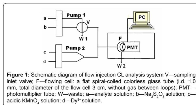
Figure 1: Schematic diagram of flow injection CL analysis system V—sampling inlet valve; F—flowing cell: a flat spiral-coiled colorless glass tube (i.d. 1.0 mm, total diameter of the flow cell 3 cm, without gas between loops); PMT—photomultiplier tube; W—waste; a—analyte solution; b—Na<sub>2</sub>S<sub>2</sub>O<sub>3</sub> solution; c—acidic KMnO<sub>4</sub> solution; d—Dy<sup>3+</sup> solution.
