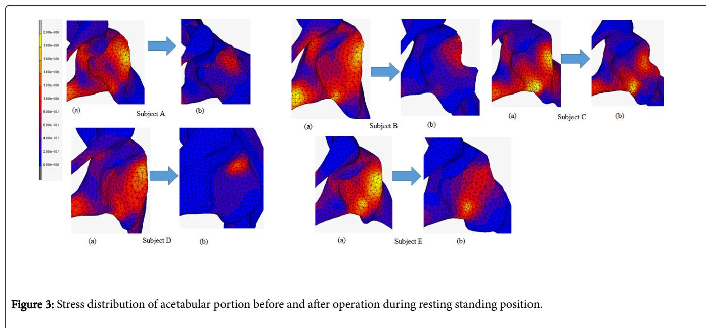
**Figure 3:** Stress distribution of acetabular portion before and after operation during resting standing position.
