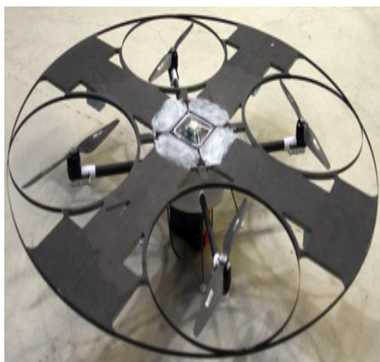
Figure 1: Prototype of AquaQuad with lower shell removed and feet attached.
