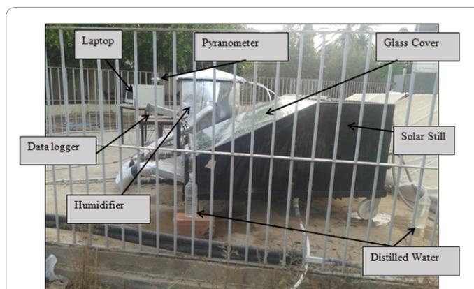
Figure 3: Photograph of the new design of solar still with an internal condenser and coupled with solar water and air heater and humidifier.
