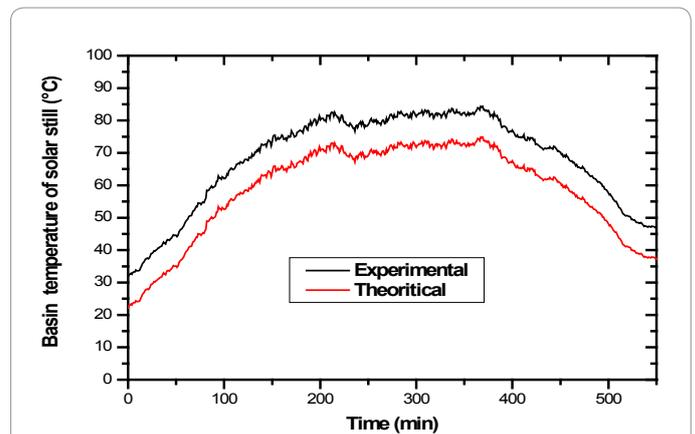
Figure 6: Comparison between numerical and experimental basin temperature of solar still.
