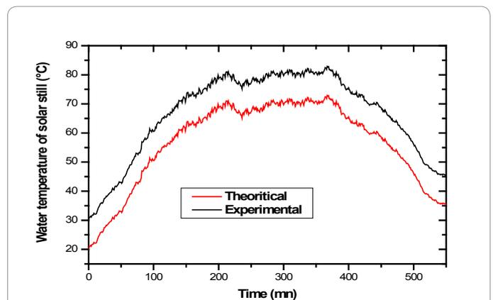
Figure 5: Comparison between numerical and experimental water temperature of solar still.
