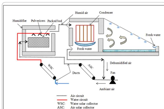
Figure 1: Schematic view of new solar distillation system the new design of solar still with an internal condenser and coupled with solar water and air heater and humidifier.
