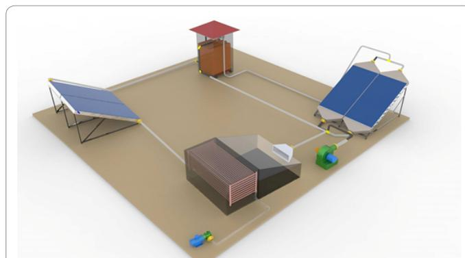
Figure 2: Three-dimensional simplified schematization of new solar distillation system by solar energy.
