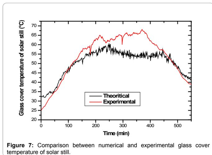
Figure 7: Comparison between numerical and experimental glass cover temperature of solar still.
