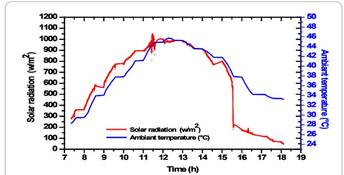
Figure 4: Solar radiation and ambient temperature measured during typical day in August.
