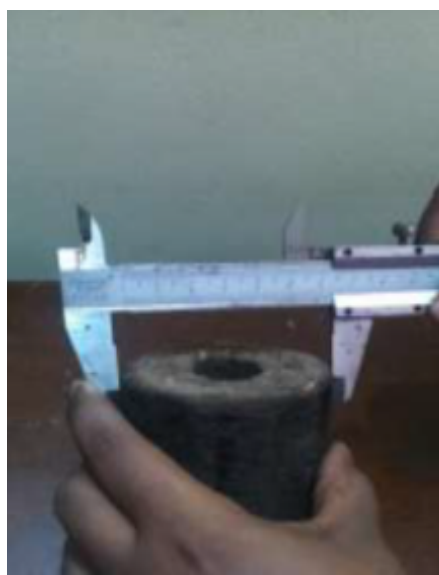
Figure 1: Measuring outer diameter of the produced briquette.
