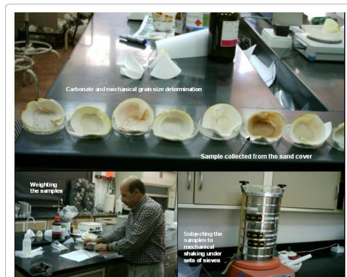
Figure 1: Preparing and processing the collected samples for petrographic and chemical analyses.
