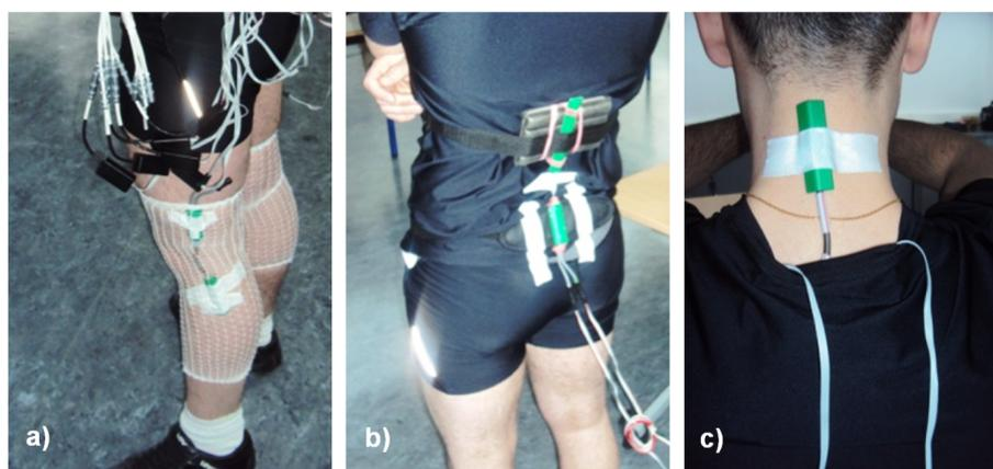
Figure 2: Placement of the goniometers on the knee (a), the lower back (b) and the neck (c).
