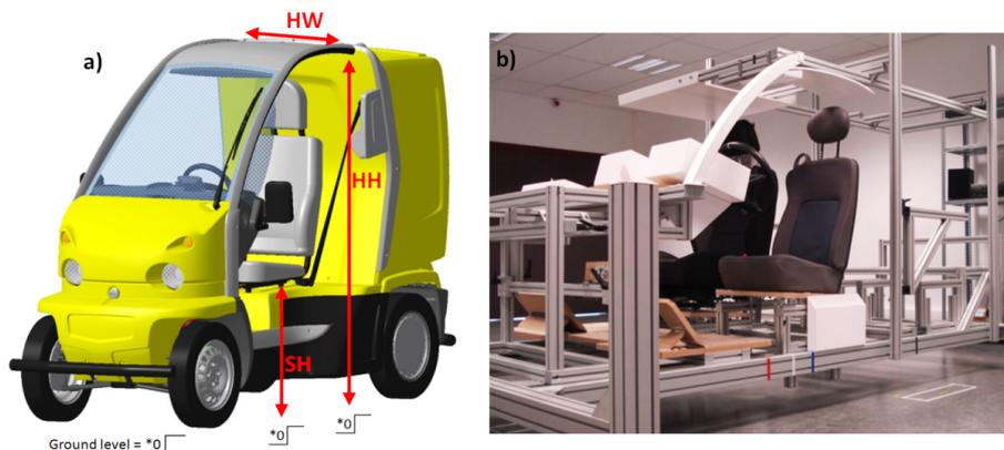
Figure 1: The future MobyPost vehicle in CAD model (a), and the multiscale physical mock-up with passenger compartment elements (b).
