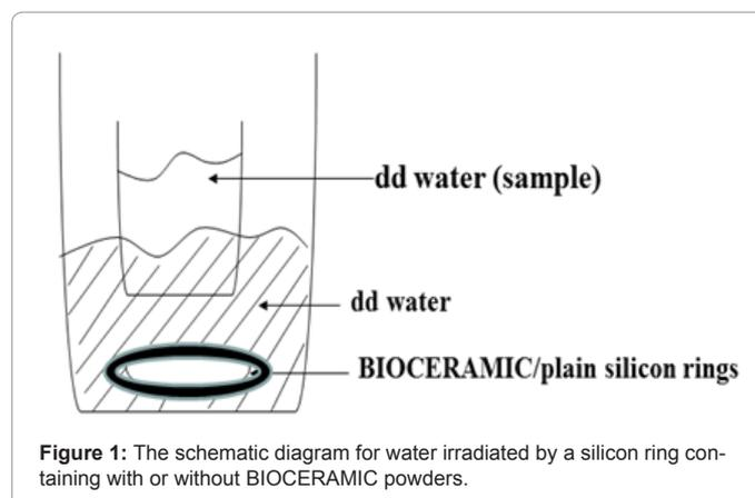
**Figure 1:** The schematic diagram for water irradiated by a silicon ring containing with or without BIOCERAMIC powders.
