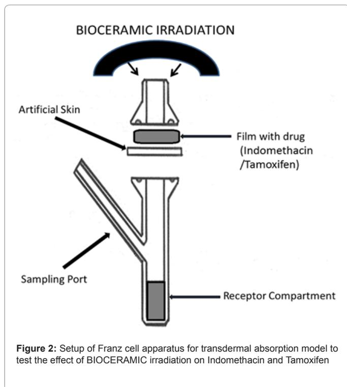
**Figure 2:** Setup of Franz cell apparatus for transdermal absorption model to test the effect of BIOCERAMIC irradiation on Indomethacin and Tamoxifen
