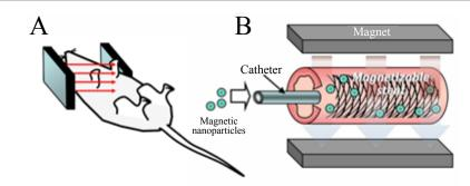
Figure 2: A targeted delivery of MNP co-formulated with Ad-Luc vectors to a deployed stent mediated by the uniform field induced magnetization effect. The uniform field generated by paired electromagnets (A) both induces high gradients on the stent and magnetizes Ad-loaded MNP, thus creating a magnetic force driving MNP to the stent struts and adjacent arterial tissue (B). (Adapted from [45] with permission).
