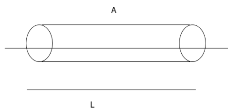
A current I flowing through a cylindrical conductor of length L and cross sectional area A
