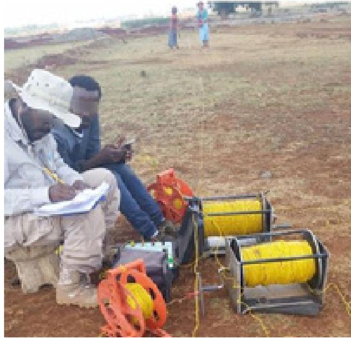
Figure 2: Electrical resistivity data acquisition on the field.
