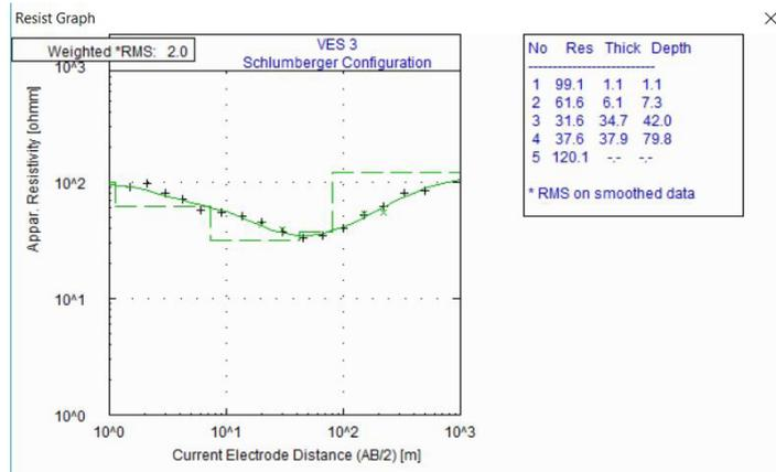
Figure 3: An interpreted VES three curves. Note: VES curve.
