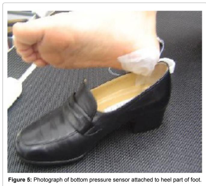
Figure 5: Photograph of bottom pressure sensor attached to heel part of foot.
