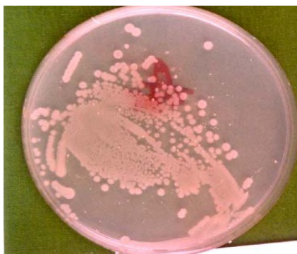
Figure 3b: Bacterial colonies in waste water sample after ultrasonic treatment at 35 KHz for 10 min.
