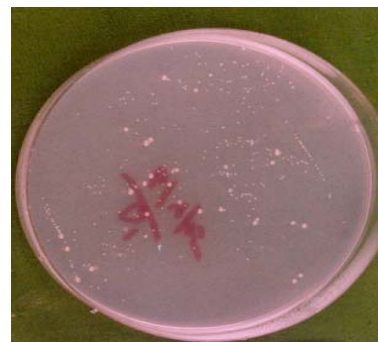
Figure 3d: Bacterial colonies in waste water sample after ultrasonic treatment at 35 KHz for 30 min.
