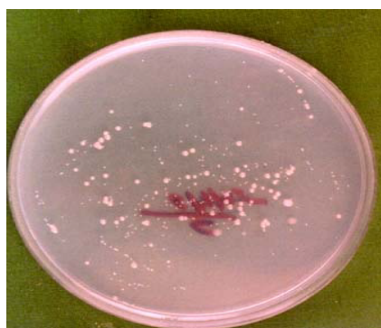
Figure 3a: Bacterial colonies in waste water sample after ultrasonic treatment at 35 KHz for 5 min.
