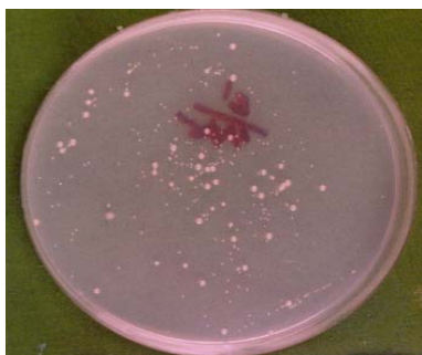
Figure 4c: Bacterial colonies in waste water sample after ultrasonic treatment at 130 KHz for 20 min.
