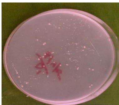
Figure 4d: Bacterial colonies in waste water sample after ultrasonic treatment at 130 KHz for 30 min.
