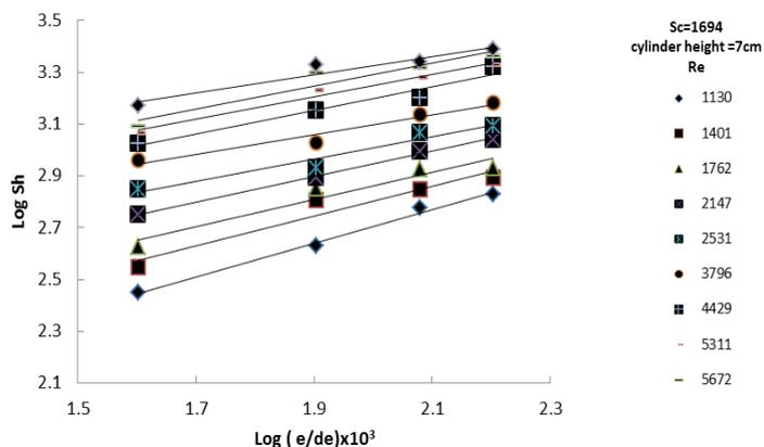
Figure 11: Effect of surface roughness (e/de) on Sh at different Re.
