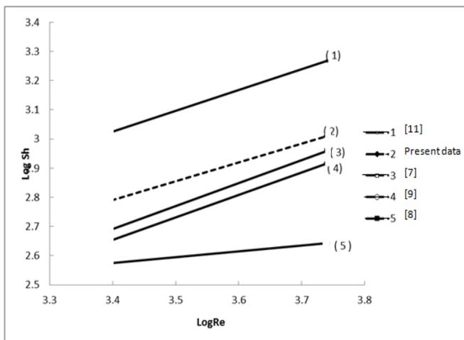
Figure 8: A comparison between the present swirl flow mass transfer data at smooth cylinder with the previous swirl flow studies.
