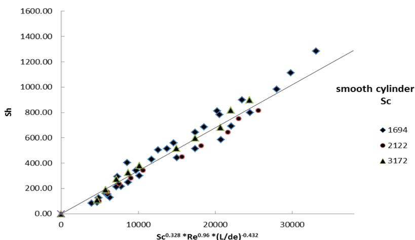
Figure 6: Overall mass transfer correlation at a smooth cylinder under swirl flow.
