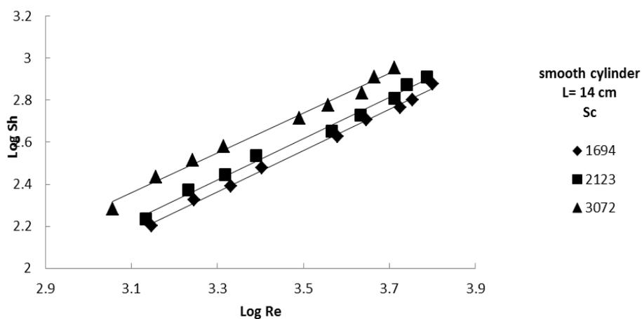
Figure 3: Effect of Re on Sh for a smooth cylinder at different Sc.
