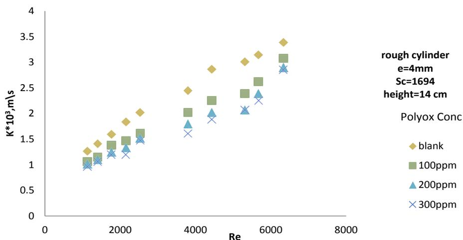
Figure 14: Effect of Re on the mass transfer coefficient at different Polyox concentration using a rough cylinder (e=4mm).
