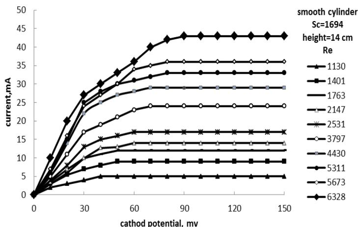
Figure 2: Typical polarization curve for smooth cylinder at different Re.
