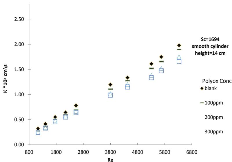
Figure 13: Effect of Re on the mass transfer coefficient at different Polyox concentration (using a smooth cylinder).
