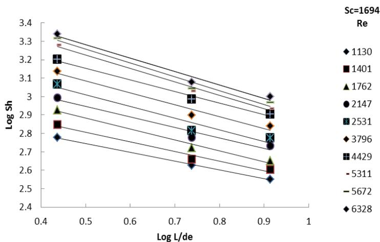
Figure 10: Effect of rough cathode cylinder height  $L/de$  on SC at different Re.
