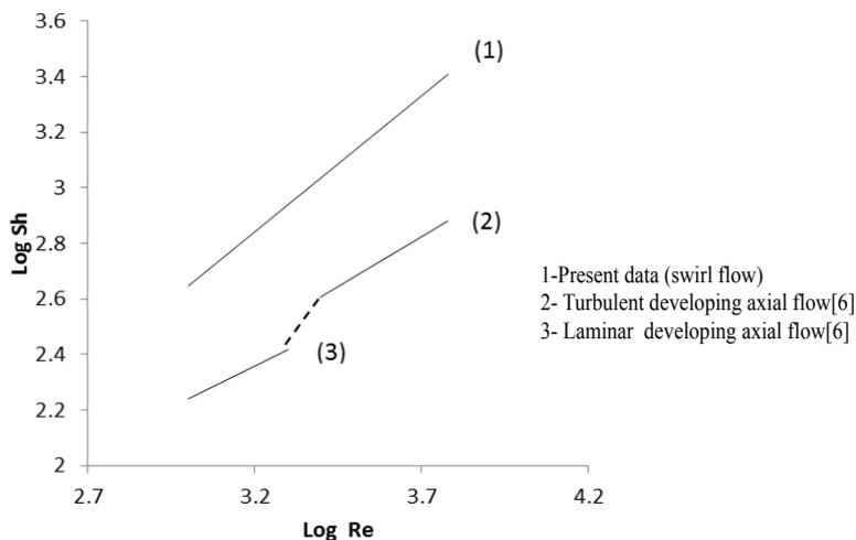
Figure 7: Comparison of the present swirl flow mass transfer coefficient with the value of axial flow in an annulus.
