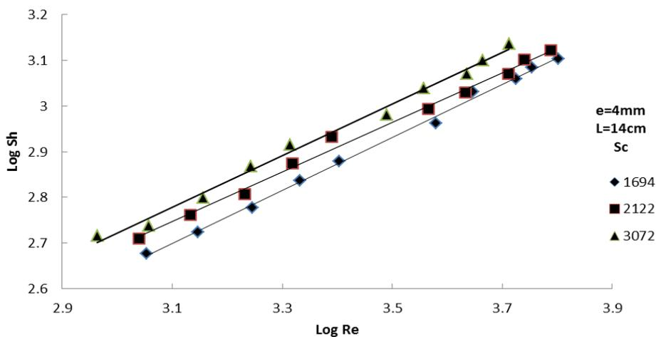
Figure 9: Effect of Re on Sh at rough cylinder ( $e=4\text{mm}$ ) for different Sc.
