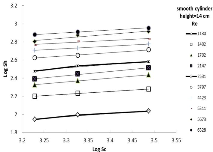
Figure 5: Effect of Sc on Sh at different Re for smooth cylinder.
