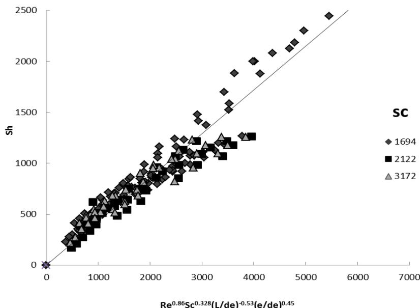
Figure 12: Overall mass transfer correlation at rough cylinders under swirl flow.
