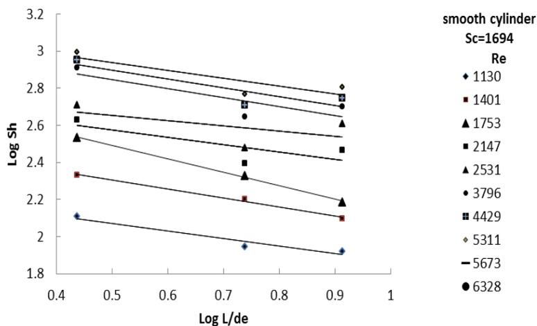
Figure 4: Effect of smooth cylinder height on Sh at different Re.
