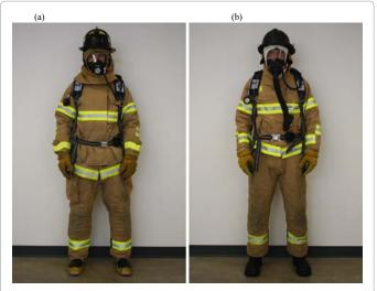
Figure 1: Two PPE configurations. (a) *Standard* PPE: helmet, heavily insulated hood, bunker style coat and pants, and rubber boots. (b) *Enhanced* PPE: lighter helmet, Nomex hood, bunker style coat and pants with reduced insulation and passive cooling system, and light weight leather/Kevlar boots.
