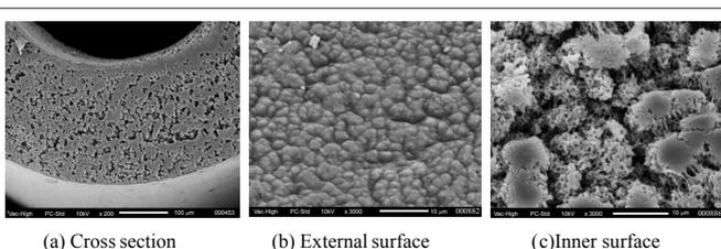
Figure 5: SEM micrographs for hollow fiber membrane prepared in 30%PVDF/65 %Triacetin/5% Glycerol cast solution. (a) Cross-section; (b) External surface; (c) inner surface.
