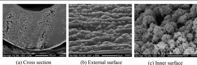
Figure 4: SEM micrographs for hollow fiber membrane prepared in 30%PVDF/70%Triacetin dope solution. (a) Cross-section; (b) External surface; (c) inner surface.
