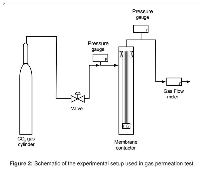
Figure 2: Schematic of the experimental setup used in gas permeation test.
