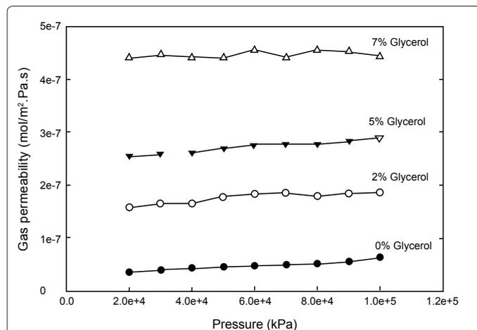
Figure 6: Gas permeability for several hollow fiber membranes prepared with different concentration of glycerol with TIPS method at Bath temperature of 25°C.
