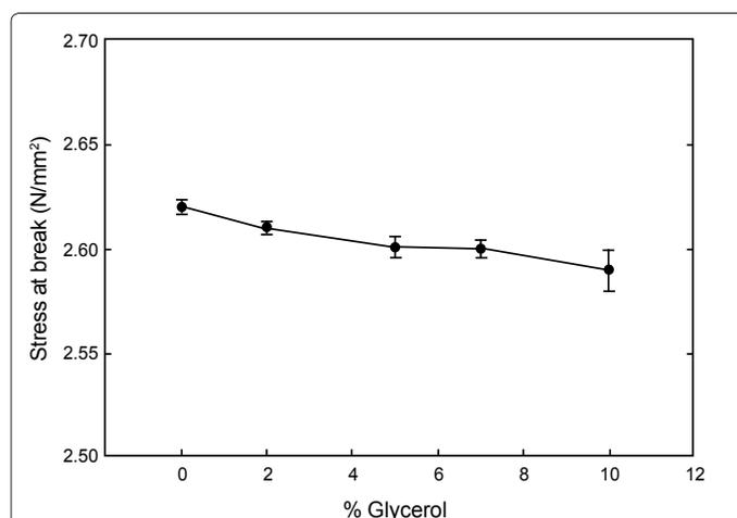
Figure 7: Membrane strength for hollow fiber membrane prepared with different glycerol concentration.
