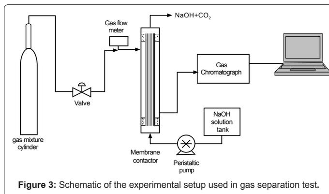
Figure 3: Schematic of the experimental setup used in gas separation test.
