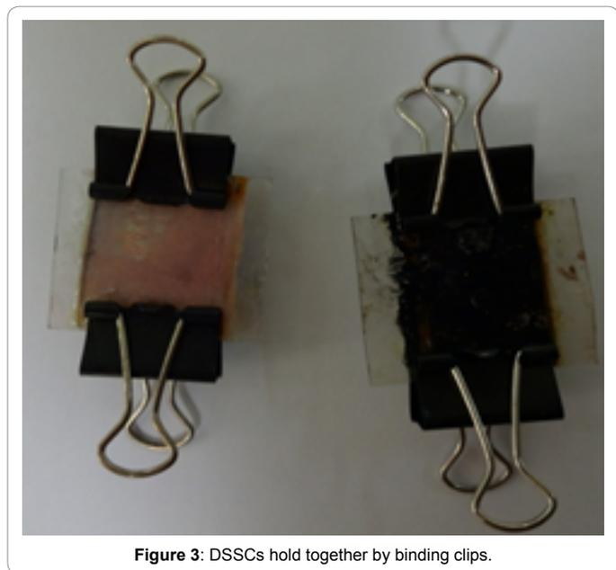
Figure 3: DSSCs held together by binding clips.
