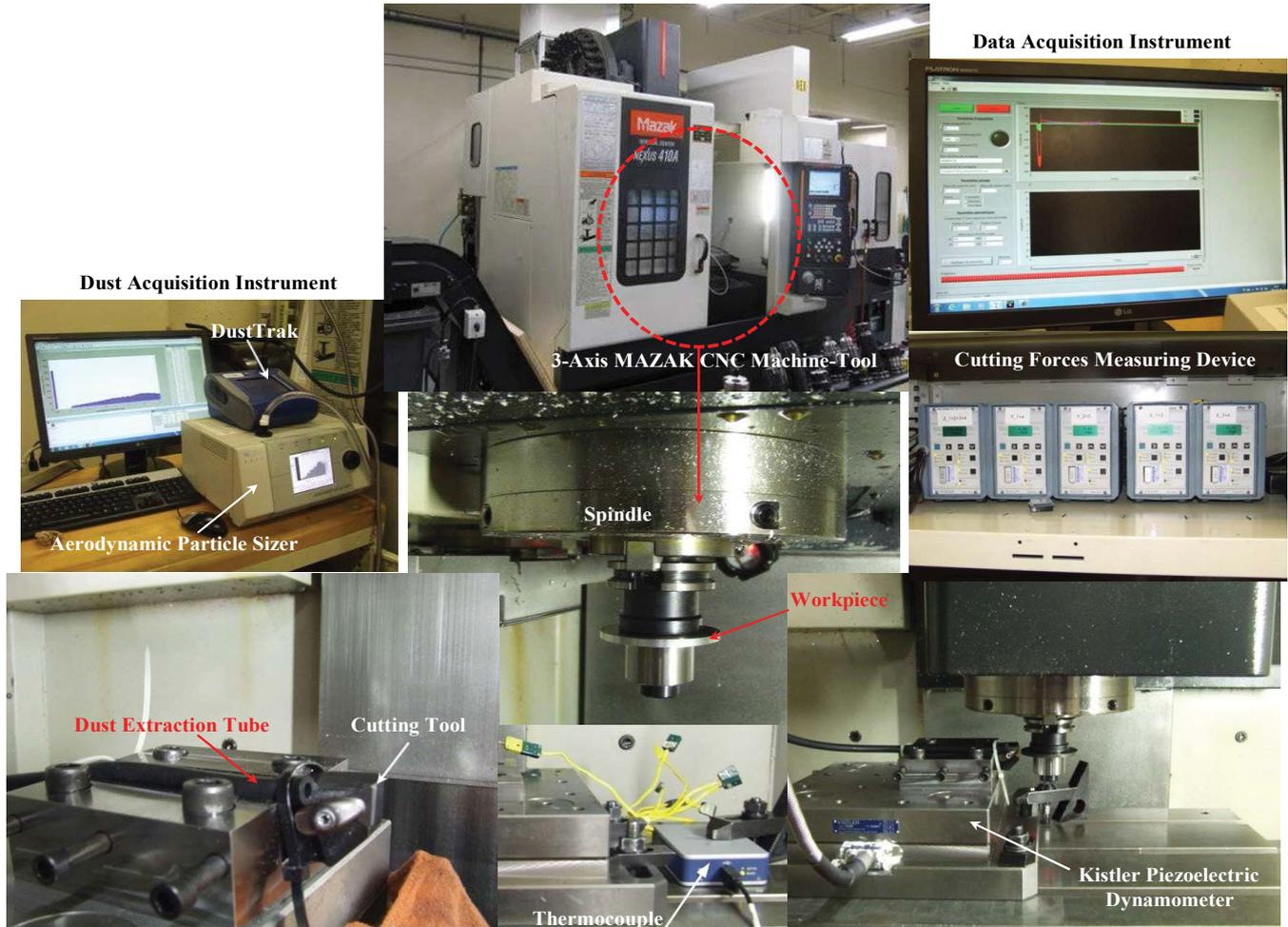
Figure 1: Experimental setup: Mazak CNC milling machine used for orthogonal cutting.
