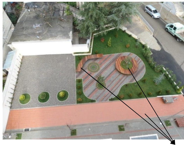
Fig 2.1.2.1: Relaxing Square. Industrial Concrete Layer, with Quartz
