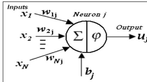
Fig.6 Information processing in a neural network unit
