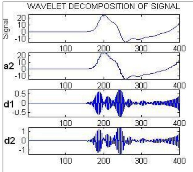
Fig. 3(a): Wavelet Decomposition of differential Inrush Current
