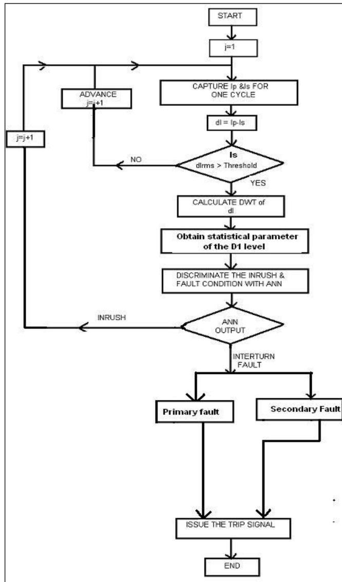
Figure 8: Flow chart for on-line discriminating scheme
