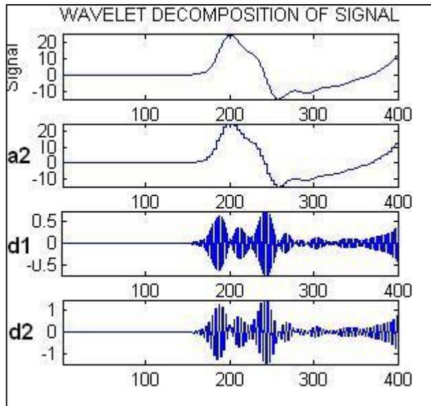
Fig. 3(c): Wavelet Decomposition of differential Current for secondary inter-turn fault
