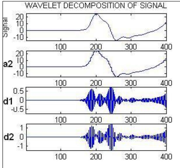
Fig. 3(b): Wavelet Decomposition of differential Current for primary inter-turn fault
