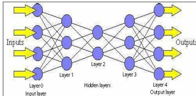
**Fig.5. Feed-forward network**
