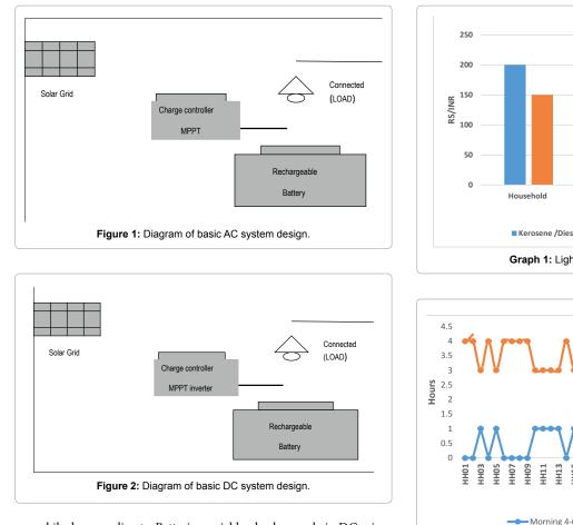
as mobile, lamp, radio etc. Batteries variable play huge role in DC micro grid system better power supply on 24 voltage with copper wiring/cable in distribution line. DC based Solar Micro-grid comparatively easy to install and can be set up by local qualified technicians with some training (Figure 2).
