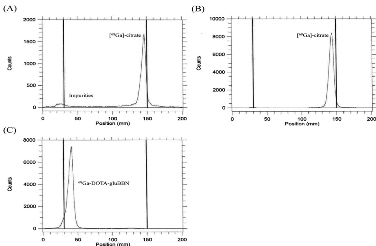
**Figure 2:** Typical iTLC profiles of eluted  $^{68}\text{Ga}$  (A), concentrated  $^{68}\text{Ga}$  solution (B), and  $^{68}\text{Ga}$ -labeled DOTA-gluBBN. The mobile phase was 0.5 M sodium citrate buffer (pH4.5). Impurities at the origin were removed by the concentration, and  $^{68}\text{Ga}$ -labelled DOTA-gluBBN was prepared by high radiochemical purity (>98%).
