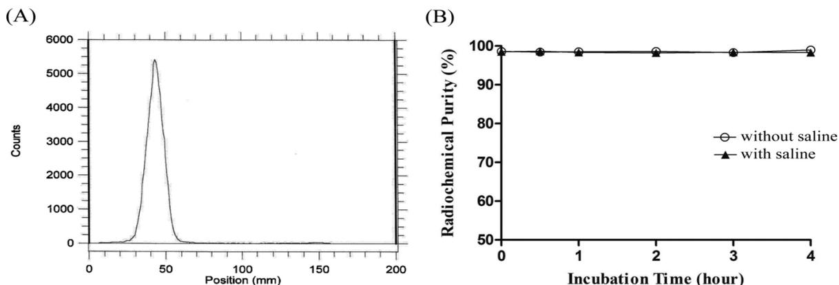
**Figure 3:** Preparation of 555 MBq of  $^{68}\text{Ga}$ -DOTA-gluBBN (A) and the stability at room temperature (B). The  $^{68}\text{Ga}$ -DOTA-gluBBN was labeled with high radioactivity over 98%, and the radiochemical purity was maintained for 4 hours.
