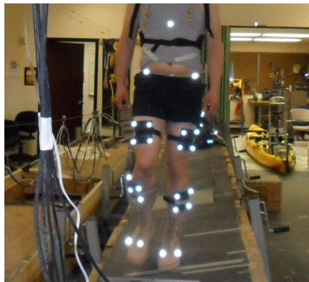
Figure 2: Participant walking back on tilted track (markers identify body and foot location so equipment can calculate center of mass and center of pressure).
