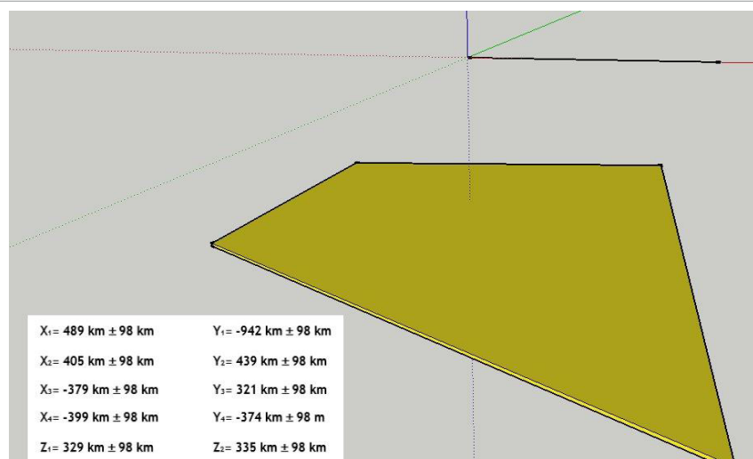
Figure 12: Computed model in Cartesian coordinates, the data have a Laplace distribution with the minimum problem being solved by the simplex method. The results are given in tabular form with the determined parameter values and their maximum error.
