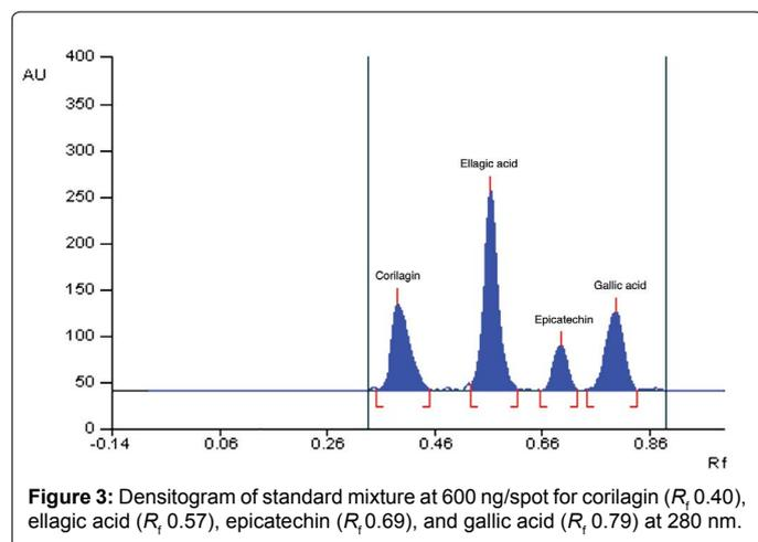
Figure 3: Densitogram of standard mixture at 600 ng/spot for corilagin ( $R_f$  0.40), ellagic acid ( $R_f$  0.57), epicatechin ( $R_f$  0.69), and gallic acid ( $R_f$  0.79) at 280 nm.
