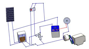
A system when solar panel is charging (Engine is stationary)
