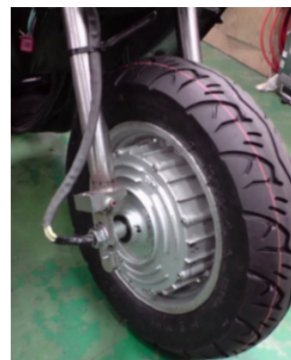
Figure 16: Hub Motor as Front Wheel Drive Unit.
