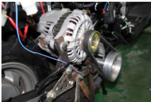
Figure 14: Generator is connected to the engine by a belt drive.
