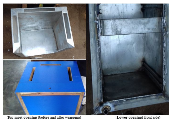
Figure 3: A photograph of our constructed refrigerator showing the openings in the different stages of the construction.
