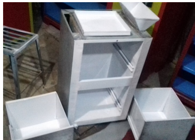
Figure 2: SS container (middle) and SS drawer chambers for food preservation.
