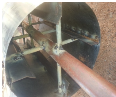
Figure 5: Plate XXVI: Shows the Baffle inside the innermost Cylinder.
