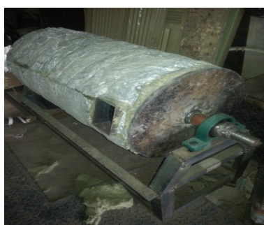
Figure 6: Plate XXVII: Insulated Cylinder of the Dryer.
