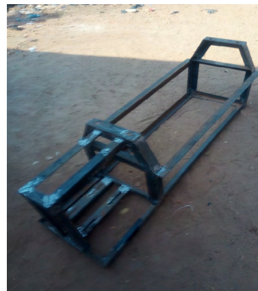
Figure 3: Plate XXIV: Frame where the dryer is mounted.
