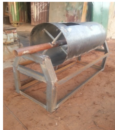
Figure 4: Plate XXV: Innermost Cylinder of the Dryer.
