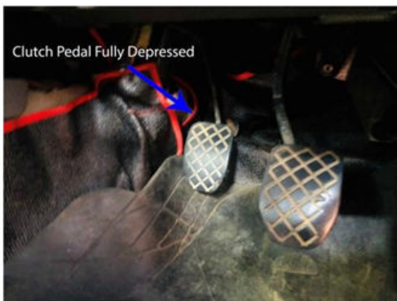
Figure5: Condition of the Clutch Pedal when touch sensor activated
