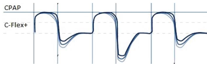
**Figure 1:** CPAP and C-Flex+ mode pressure curves over time [21]. The curves do show three subsequent inspirations and expirations. At the beginning of each expiration the particular relief drop in pressure is clearly observed.
