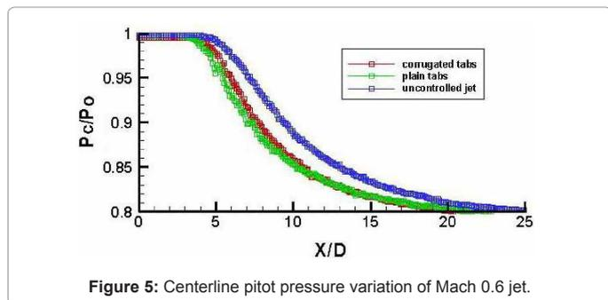
Figure 5: Centerline pitot pressure variation of Mach 0.6 jet.
