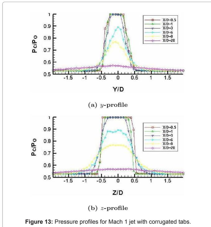
reduction caused by the plain tabs is larger than that by the corrugated tabs, at all the Mach numbers studied. Up to an axial distance of about  $22D$ , the uncontrolled and controlled jets retain their signatures. For the sonic jet, a maximum core length reduction of 32.3% is achieved with the plain tabs, whereas with the corrugated tabs the core length reduction is 17.63%. At all subsonic Mach number and sonic Mach number of the present study, the difference between the core length
