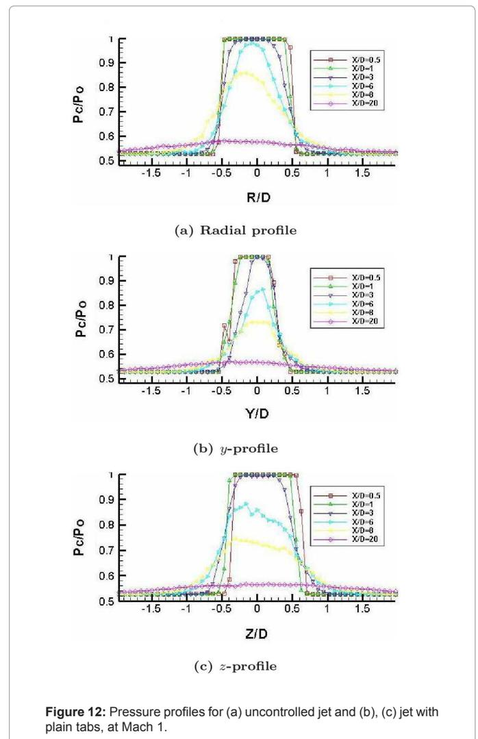
Figure 12: Pressure profiles for (a) uncontrolled jet and (b), (c) jet with plain tabs, at Mach 1.
