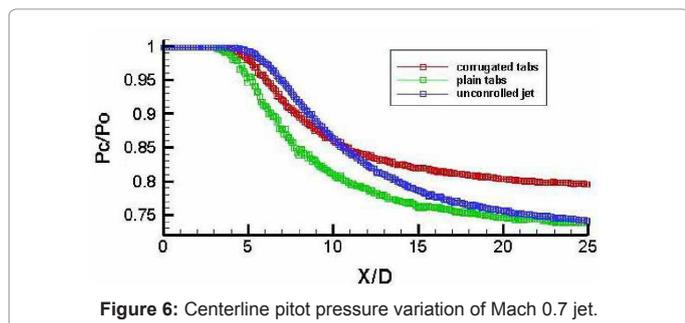
Figure 6: Centerline pitot pressure variation of Mach 0.7 jet.
