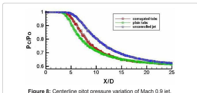
Figure 8: Centerline pitot pressure variation of Mach 0.9 jet.
