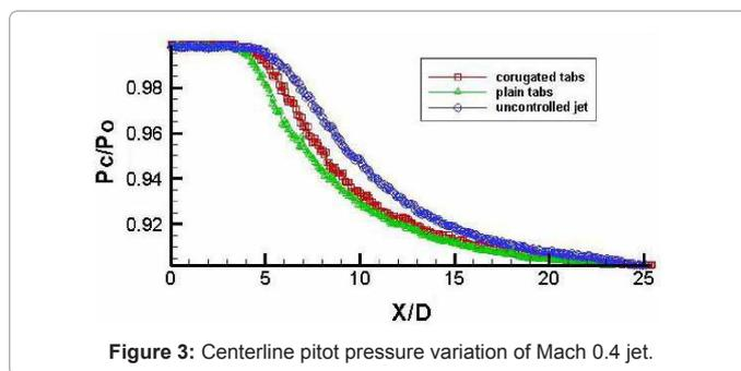
Figure 3: Centerline pitot pressure variation of Mach 0.4 jet.
