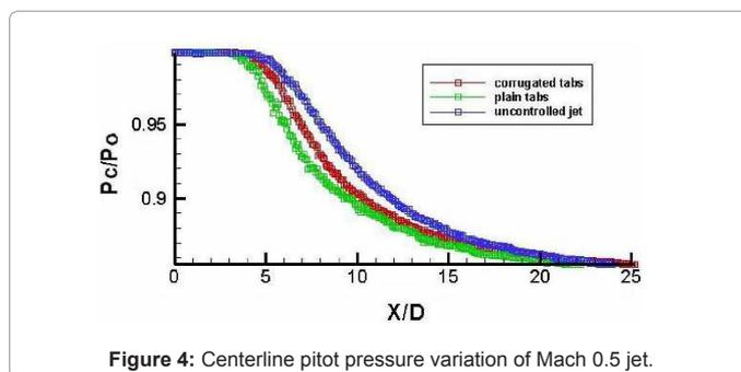
Figure 4: Centerline pitot pressure variation of Mach 0.5 jet.
