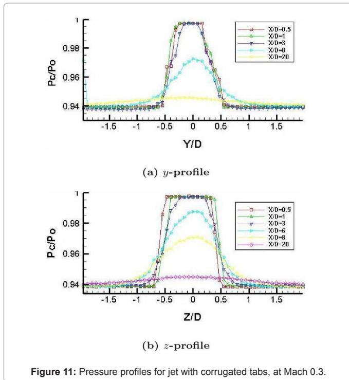
Figure 11: Pressure profiles for jet with corrugated tabs, at Mach 0.3.
