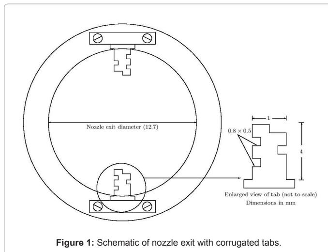
Figure 1: Schematic of nozzle exit with corrugated tabs.
