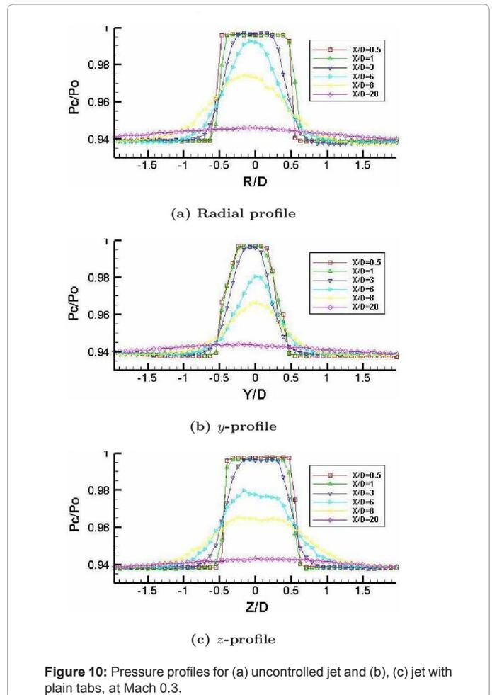
Figure 10: Pressure profiles for (a) uncontrolled jet and (b), (c) jet with plain tabs, at Mach 0.3.
