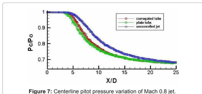
Figure 7: Centerline pitot pressure variation of Mach 0.8 jet.
