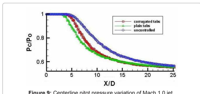
Figure 9: Centerline pitot pressure variation of Mach 1.0 jet.
