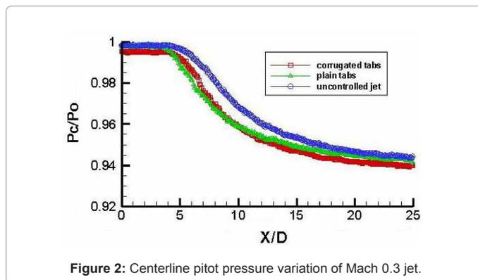
Figure 2: Centerline pitot pressure variation of Mach 0.3 jet.
