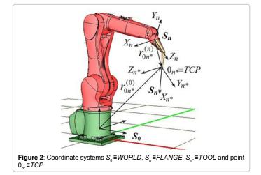
of the relative rotation of the links connected by them. The tool can be rigidly attached to the last link of the industrial robot manipulation system. For this purpose, the connecting flange is provided in the design of the last link. In Figure 1, the connecting flange is depicted in the form of a disk, inside of which there is a hinge with the rotation axis perpendicular to the plane of the disk.
