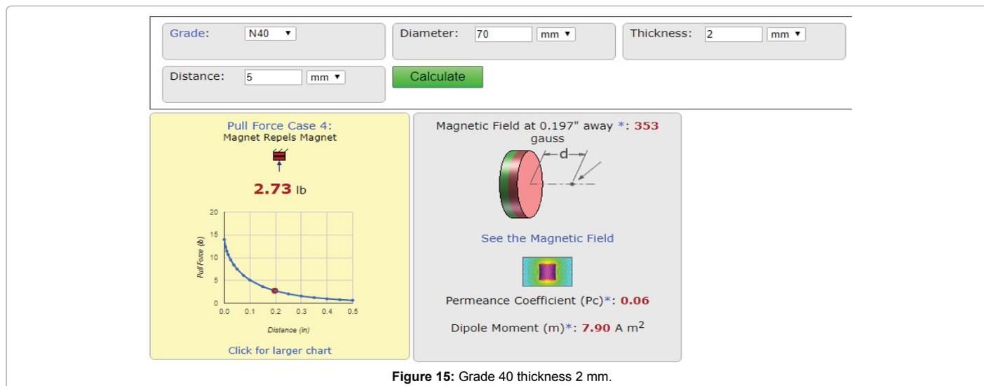
Figure 15: Grade 40 thickness 2 mm.
