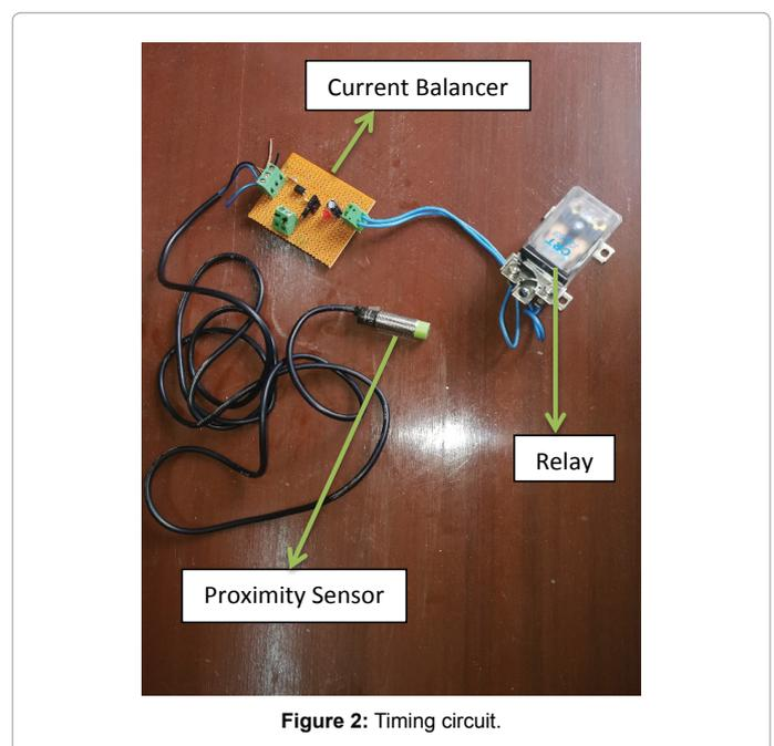
Figure 2: Timing circuit.
