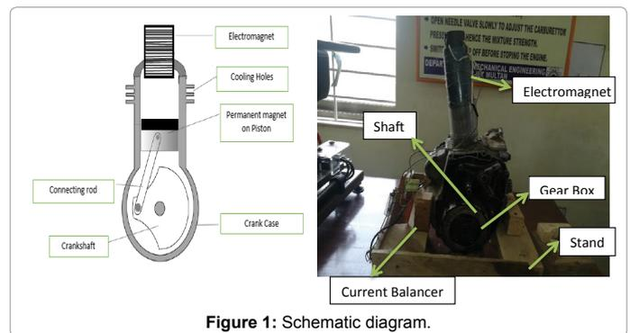
Figure 1: Schematic diagram.
