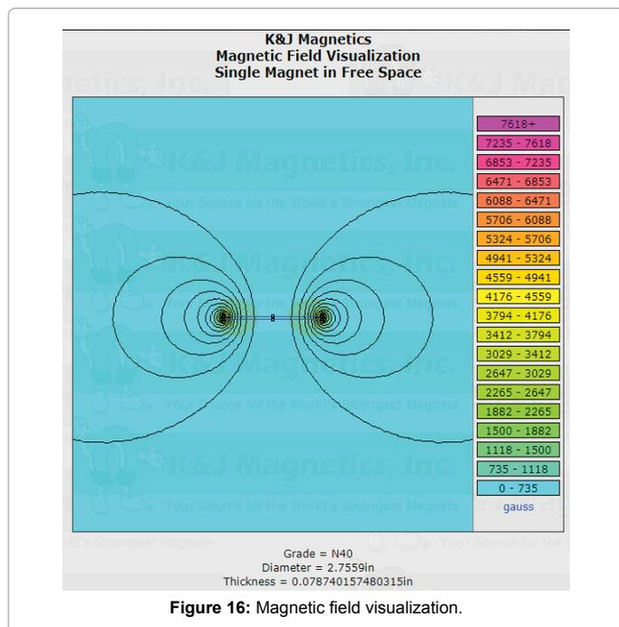
Figure 16: Magnetic field visualization.
