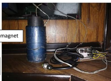
Figure 8: Electromagnet with relay.
