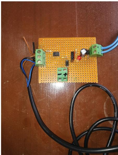
Figure 3: Current balancer circuit.
