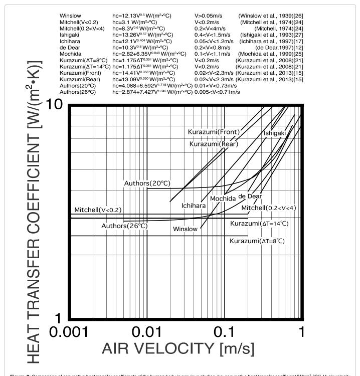
Figure 2: Comparison of convective heat transfer coefficients of the human body in previous studies. hc: convective heat transfer coefficient [W/(m²-°C)]. V: air velocity [m/s]. ΔT: difference between mean skin temperature and air temperature [°C].
