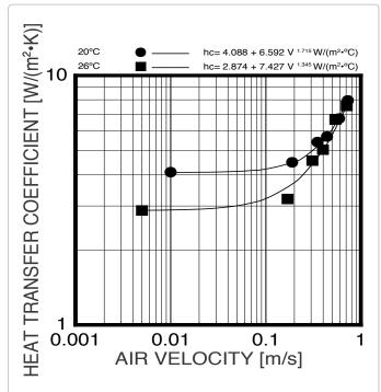
Figure 1: Relation between heat transfer coefficients and air velocity. hc: convective heat transfer coeffi-cient [W/(m²-o°C)]. V: air velocity [m/s].
