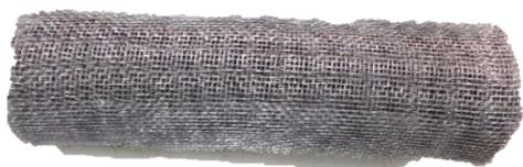
Figure 11: Wire mesh filled with charcoal.
