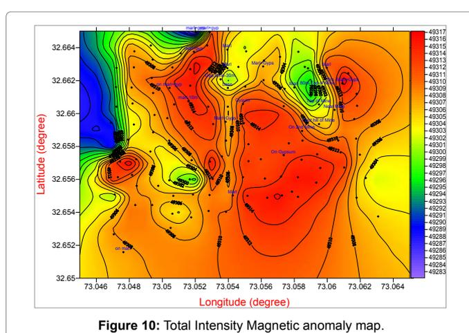
magnetic lows represent the anomalous zones where the existence of probable salt dome has been identified.
