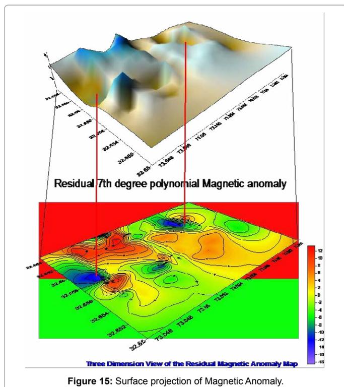
existence of salt dome is delineated. Similarly, in three dimension surface of magnetic map (Figure 15), magnetic lows represent the anomalous zones where the existence of probable salt dome has been identified.
