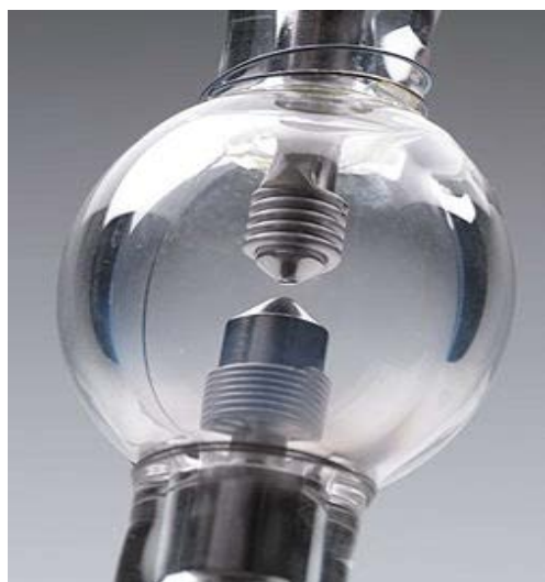
Plate 2: Xenon lamp as a continuous radiation source (Source: McCarthy [62]).
