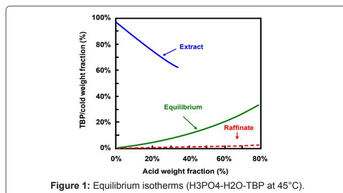
Figure 1: Equilibrium isotherms ( $H_3PO_4$ - $H_2O$ -TBP at 45°C).
