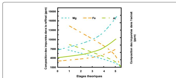
Figure 10: Raffinate and extract impurities' contents along the ideal extractors for MIBK+TBP.
