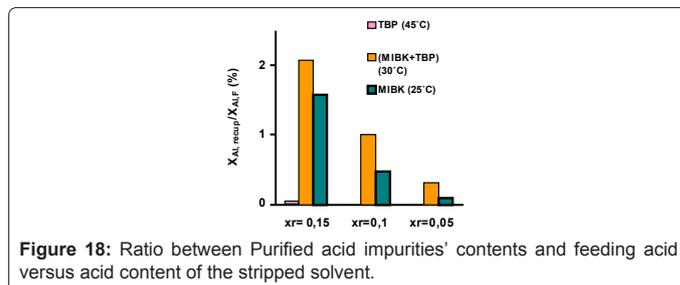
Figure 18: Ratio between Purified acid impurities' contents and feeding acid versus acid content of the stripped solvent.
