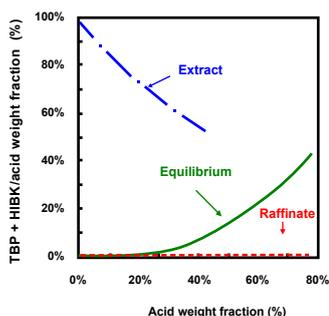
Figure 3: Equilibrium isotherms (H<sub>3</sub>PO<sub>4</sub>-H<sub>2</sub>O- TBP+MIBK at 30°C).
