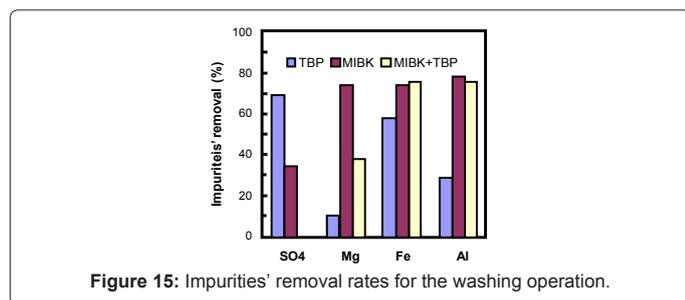
Figure 15: Impurities' removal rates for the washing operation.
