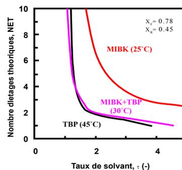
Figure 6: Number of theoretical stages for extracting H<sub>3</sub>PO<sub>4</sub> from the WPA versus the solvent rate.
