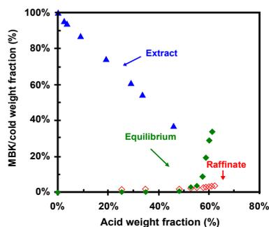
Figure 2: Equilibrium isotherms (H<sub>3</sub>PO<sub>4</sub>-H<sub>2</sub>O-MIBK at 25°C).
