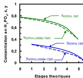
Figure 7: Raffinate and extract acid contents along the ideal extractors.
