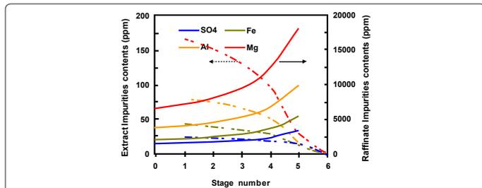
Figure 8: Raffinate and extract impurities' contents along the ideal extractors for TBP.
