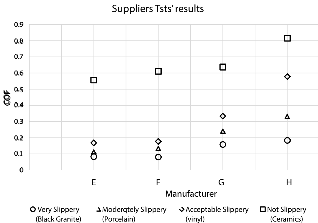
Figure 3: Tests' results performed by the suppliers in order to validate their tribometers.
