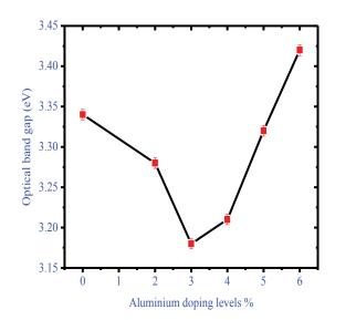
Figure 5: Variation of optical band gap for ZnO:Al with various doping levels of Aluminum (%).
