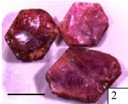
Figure 2: Basal sections of corundum grains. Scale: 5 mm.
