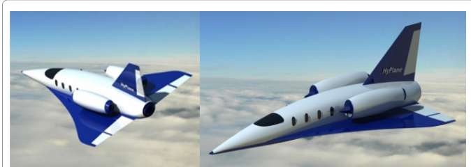
Figure 2: Low wing loading aerodynamic configuration.
